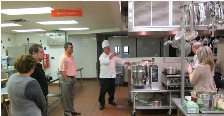
*A demonstration of how the steam jacketed kettle is used and how it benefits commercial foodservice operators was performed for representatives from GTI and Oklahoma Natural Gas.*
