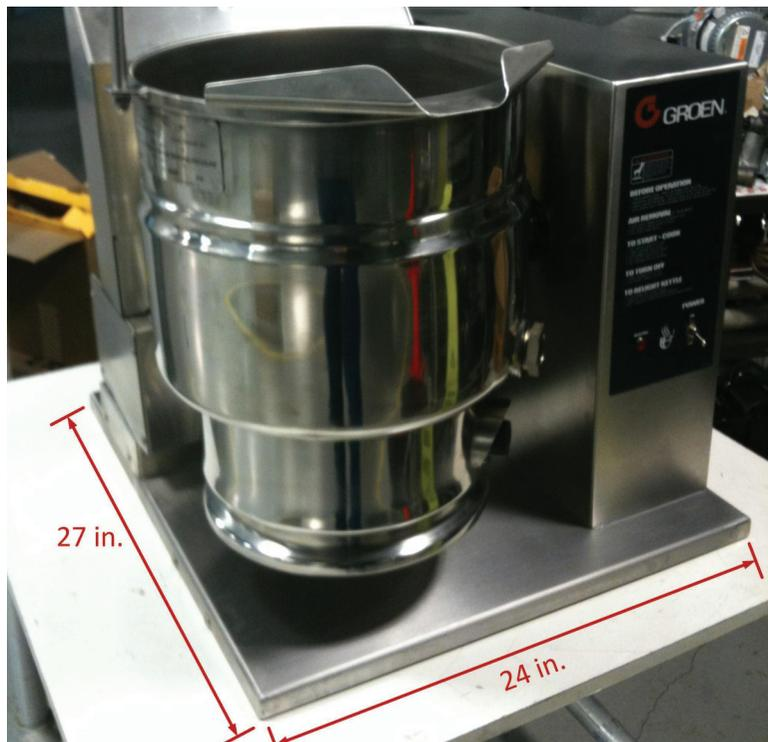
*The steam jacketed kettle was tested at the GTI lab in accordance with ASTM standards to determine Maximum Energy Input Rate, Heatup Efficiency and Rate, Production Capacity, and the Simmer Rate.*
