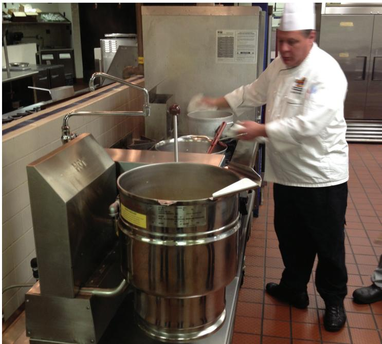
*As part of this commercial foodservice research project, the chef demonstrated the advantages of a steam jacketed kettle compared with using a stock pot on a range.*
